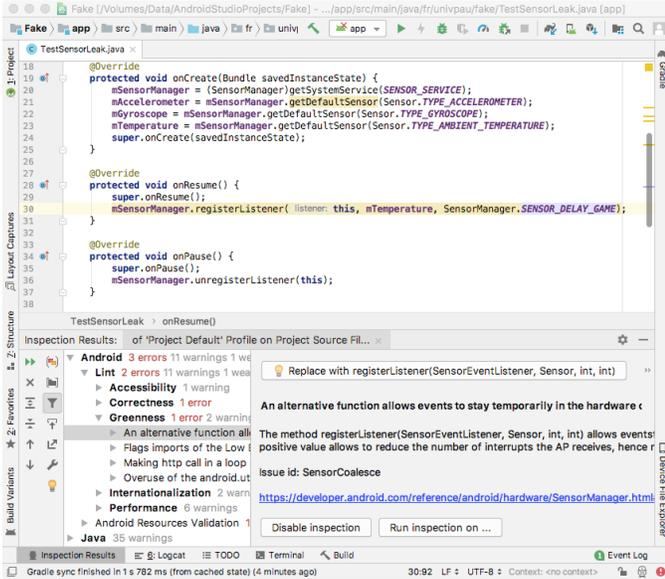
Fig. 2. Defect highlighting for the green bug *SensorCoalesce*.
